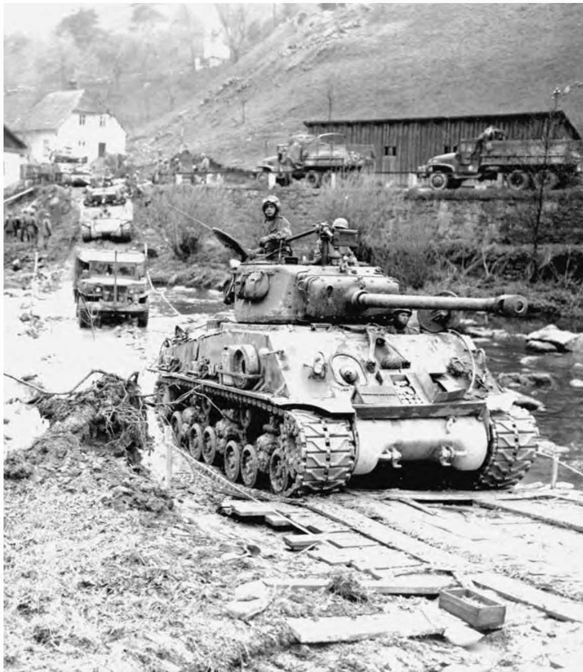
TANKS AND TRUCKS of a Third Army armored division fording a stream during their advance into Austria. In the foreground is a medium tank M4A3 (76-mm. long-barrel gun with muzzle brake) with horizontal volute spring suspension and an improved, wider track measuring twenty-three inches.
