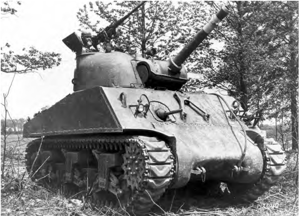
TWO TYPES OF U. S. TRACKED VEHICLES, each mounting a 105-mm. howitzer. 105-mm. howitzer motor carriage M7 (top); medium tank M4A3 with 105-mm. howitzer (bottom).
