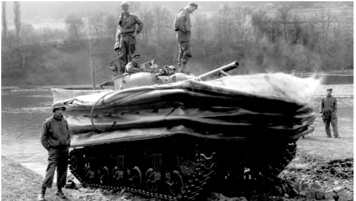
A DUPLEX-DRIVE TANK (DD tank), with its flotation device raised, entering the water (top); flotation device after being lowered (bottom). The canvas flotation device made the tank vulnerable to mines and objects floating in the water.
