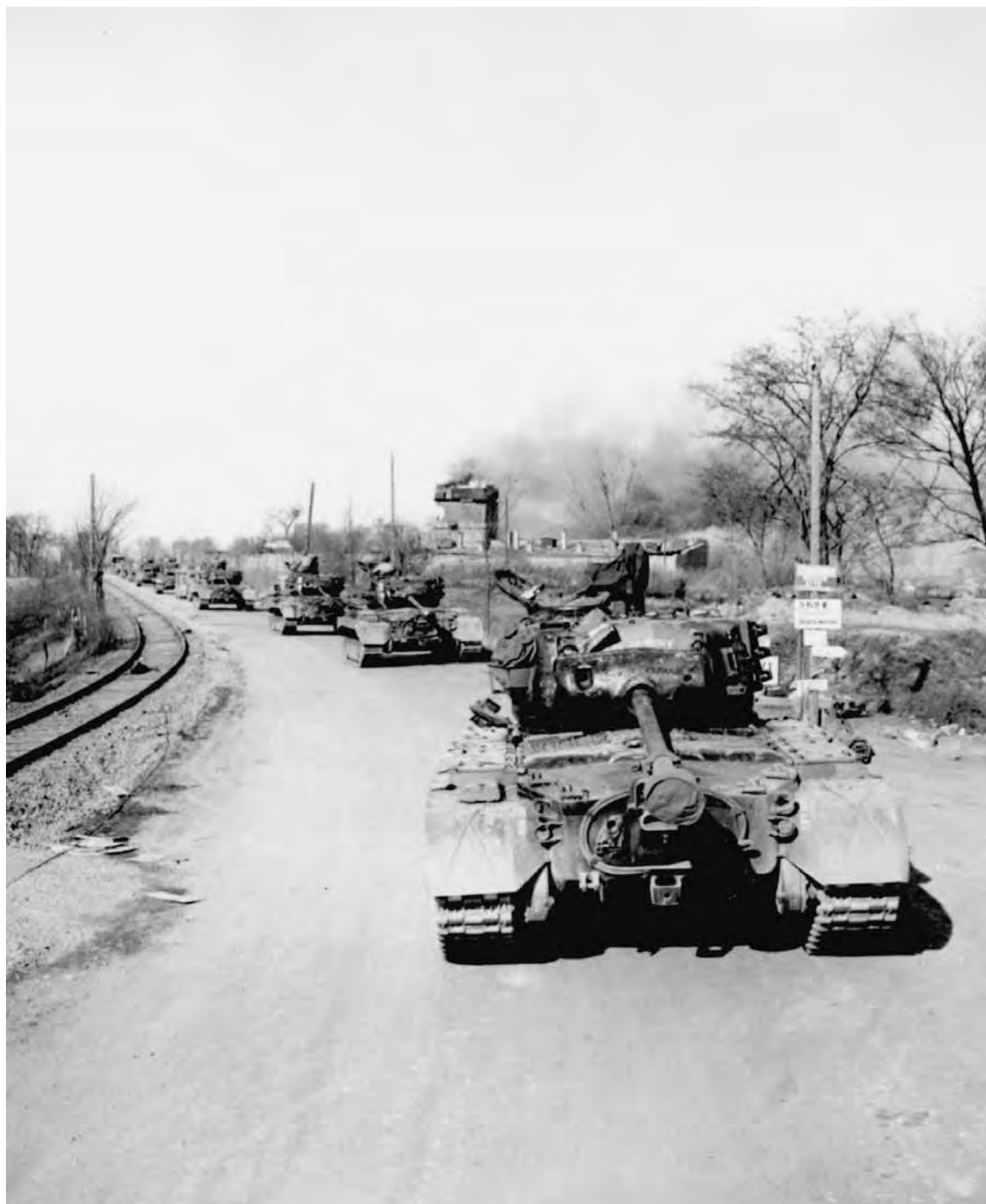
MEDIUM TANKS M26 moving through Wesel on the way to the front.
