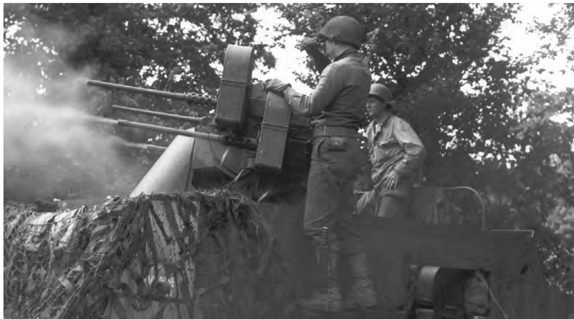
MULTIPLE GUN MOTOR CARRIAGE M16 with its four .50-caliber machine guns firing at the enemy in support of an infantry advance (top). This vehicle was a weapon of an antiaircraft artillery unit, but the lack of enemy air activity in Normandy made possible its use in other roles. U. S. artillerymen emplacing a 155-mm. howitzer M1 in a camouflaged position (bottom).
