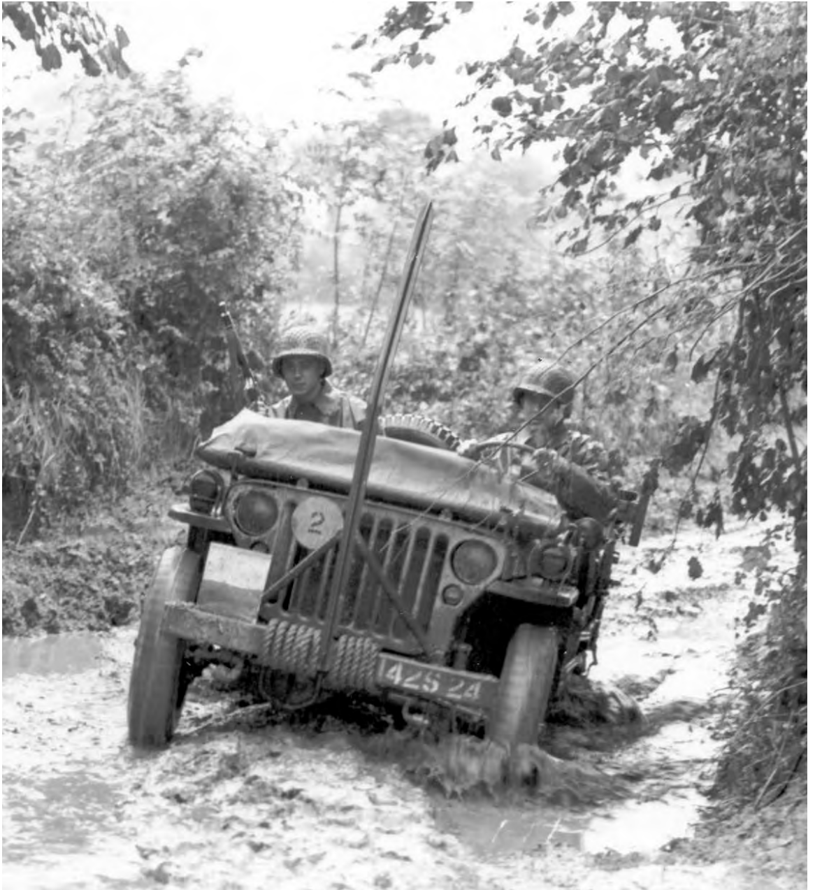
JEEP SPLASHING THROUGH A FLOODED ROAD IN NORMANDY. The rains, which held up the advance, flooded the dirt roads which by this time were in a bad state of repair from the heavy traffic and shelling. On the front of the jeep is an iron bar used to cut thin strands of wire that the enemy strung across the roads level with the heads of the occupants of vehicles, which traveled with tops and windshields down.
