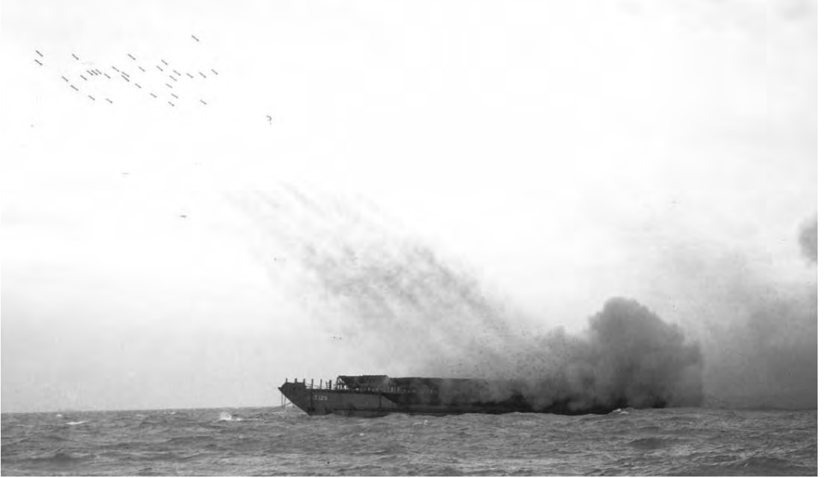
LCT(R) FIRING ROCKETS DURING A TEST in Portsmouth Harbor, England (top). Close-up of the rocket launchers (bottom). These ships converted from landing craft, tank, were equipped to fire as many as 1,000 rockets.
