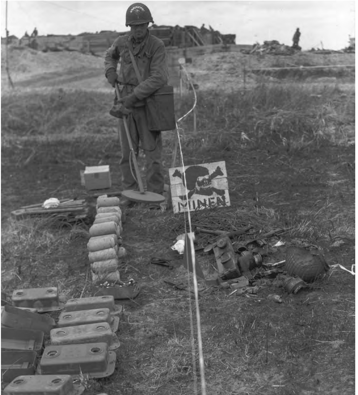
A MEMBER OF AN ENGINEER UNIT using a mine detector SCR 625. The ground outlined with white tape had not been cleared of enemy mines and enemy signs were used to mark the mined areas. Army and Navy demolition teams, following the assault infantry, found the beach less thickly obstructed than expected, and Utah Beach was cleared in an hour. Engineers prepared exits from the beach by clearing lanes through the mine fields.
