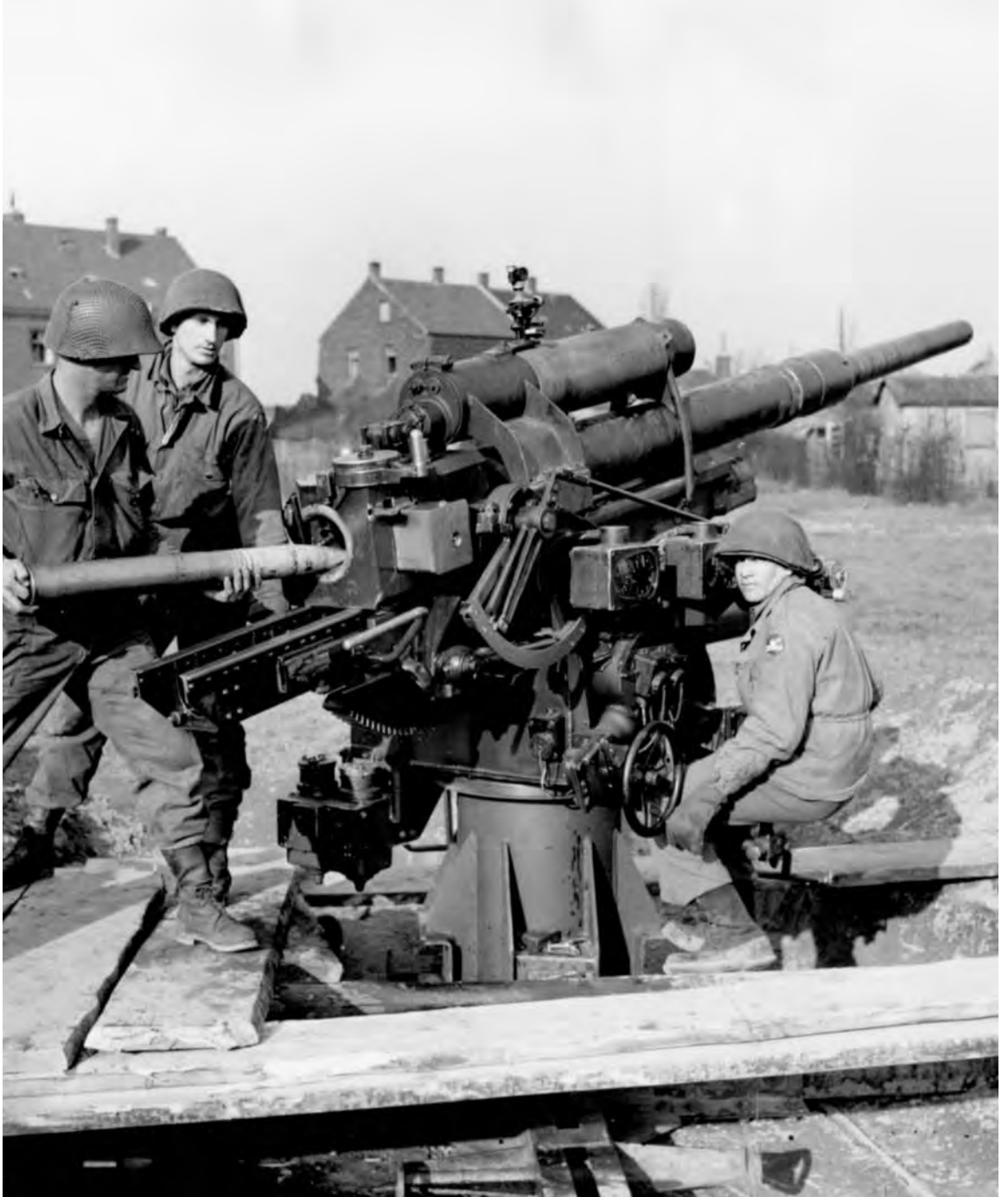
A THREE-MAN ARTILLERY CREW preparing to fire a multipurpose 88-mm. gun captured in Germany.
