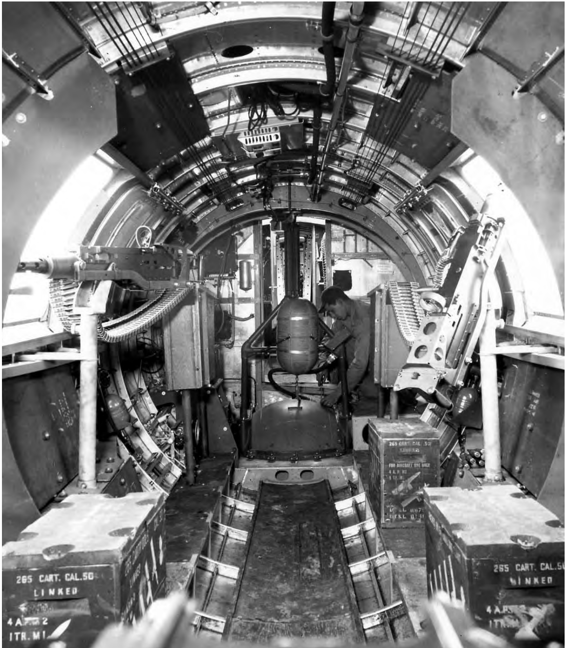
INTERIOR OF A B-17 showing two .50-caliber Browning machine guns. These planes were highly complex machines, well armed, with machine guns in front, rear, sides, top, and bottom. The man in the picture is working on the gun turret which protruded beneath the fuselage. The tank on top of this turret was for oxygen.
