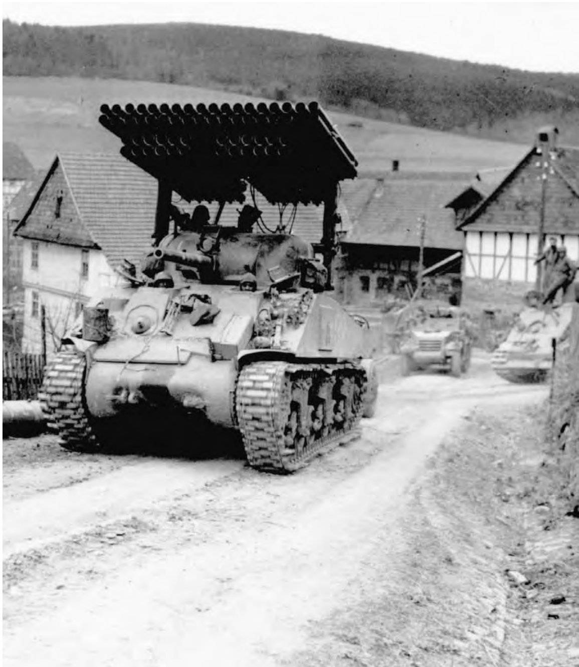
4.5-INCH MULTIPLE ROCKET LAUNCHER T34 mounted on a medium tank. The Germans stubbornly defended the industrial area of the Ruhr even though an army group was caught in the trap with little hope of escape. On the Allied flanks, advances were made as the enemy began to disintegrate.
