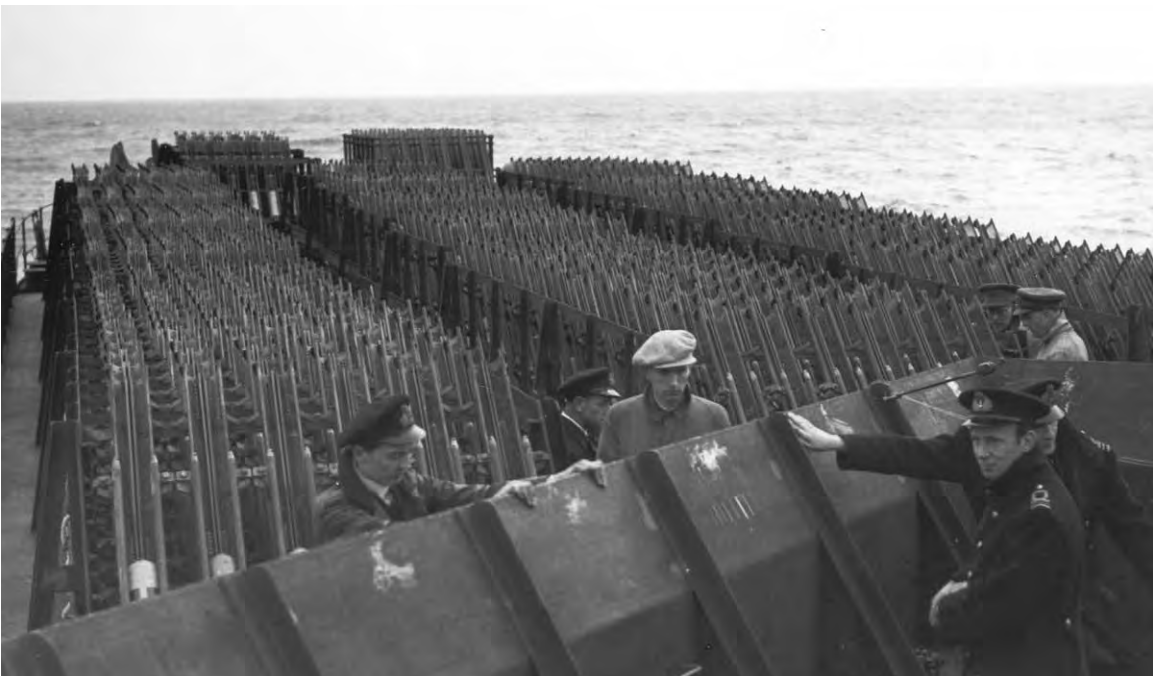
LCT(R) FIRING ROCKETS DURING A TEST in Portsmouth Harbor, England (top). Close-up of the rocket launchers (bottom). These ships converted from landing craft, tank, were equipped to fire as many as 1,000 rockets.
