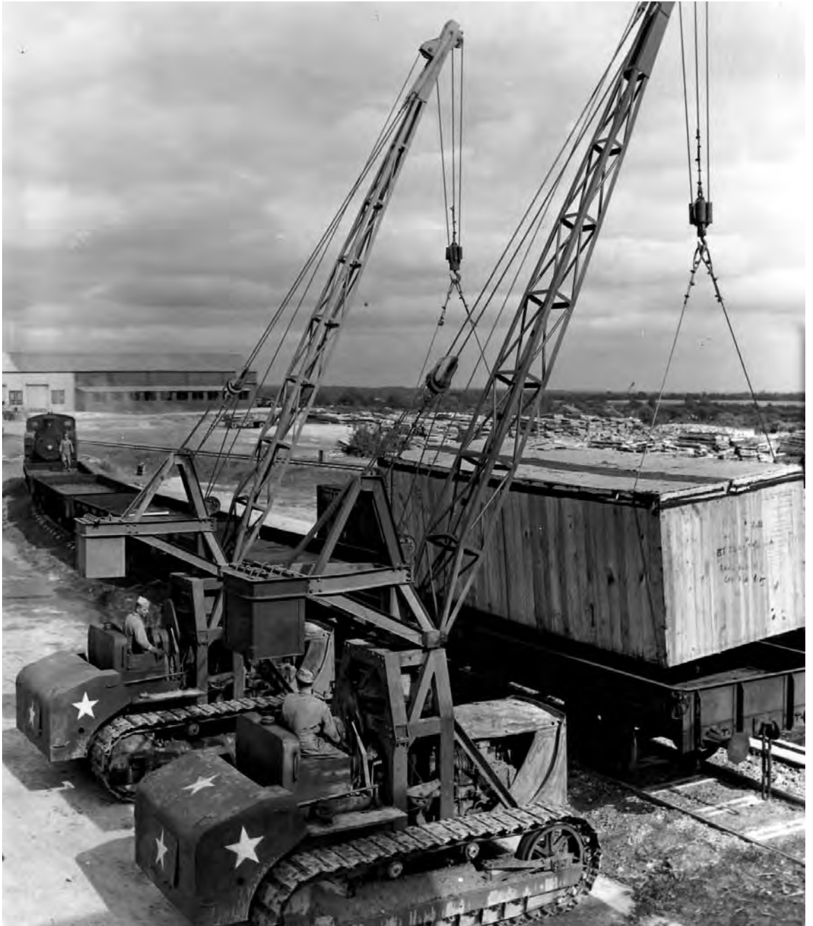
ENLISTED MEN OF THE ORDNANCE DEPARTMENT operating caterpillar tractor cranes to unload a crated gun carriage (half-track) which weighed approximately 20,000 pounds. The Ordnance Department maintained a large depot at Tidworth, England.
