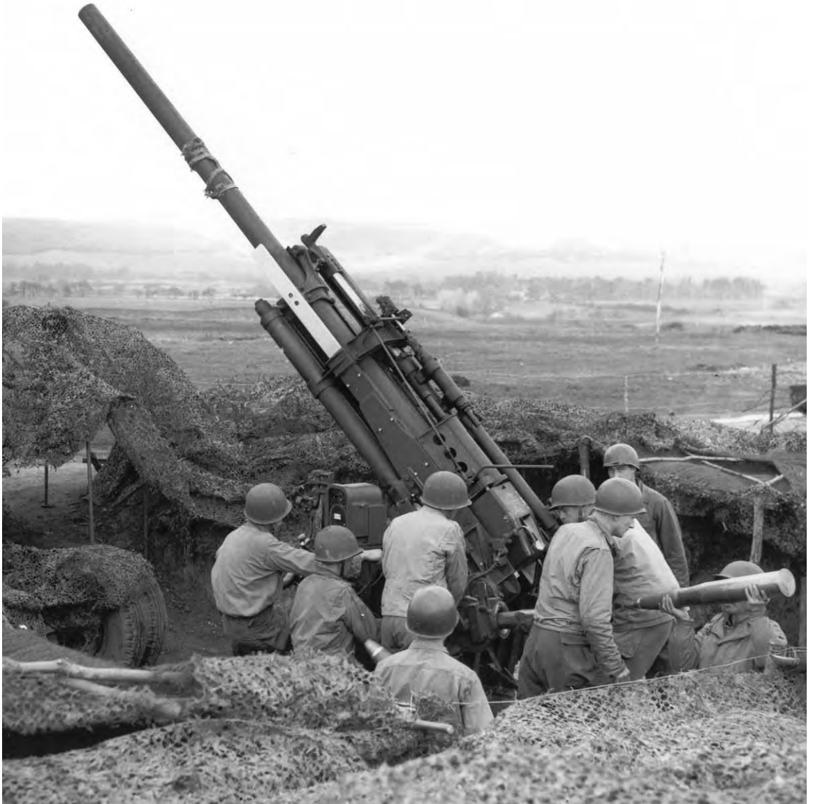
GUN CREW OF AN ANTI-AIRCRAFT ARTILLERY GROUP operating a 90-mm. gun M1 near the coast of England, April 1944. In order to cope with the latest developments in the fields of high-altitude bombing, a 90-mm. anti-aircraft gun with longer range, greater muzzle velocity, and a larger effective shell-burst area was introduced.
