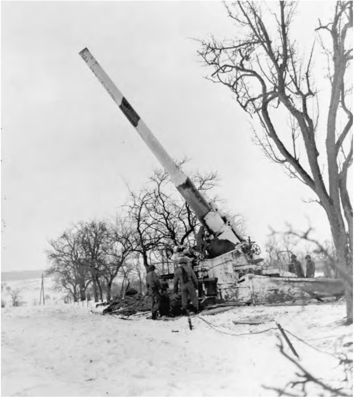
A CAMOUFLAGED 8-INCH GUN M1 located in the southern portion of the Third Army zone. This gun was capable of firing a 240-pound projectile a distance of 20 miles. The troops left in this area were placed on the defensive during the fighting in the Ardennes sector. Heavy artillery in the area fired on enemy installations in the triangle of the Moselle and Saar Rivers and West Wall fortifications.
