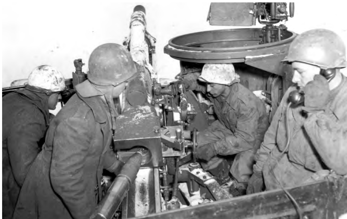
LOADING A 105-MM. SHELL into the howitzer of a Priest (top); snow on the camouflage net over a 155-mm. howitzer M1 helps conceal its position (bottom).
