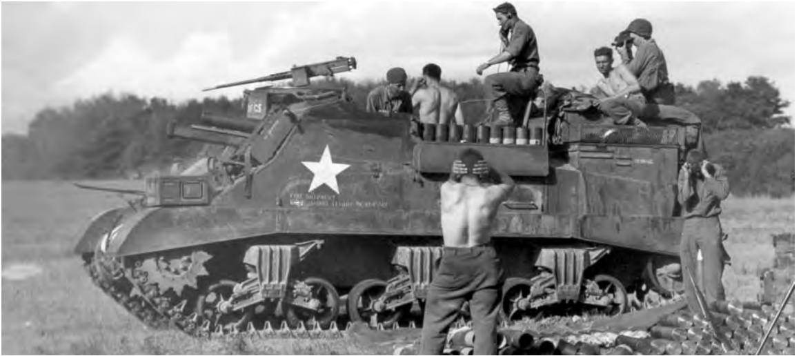
TWO TYPES OF U. S. TRACKED VEHICLES, each mounting a 105-mm. howitzer. 105-mm. howitzer motor carriage M7 (top); medium tank M4A3 with 105-mm. howitzer (bottom).
