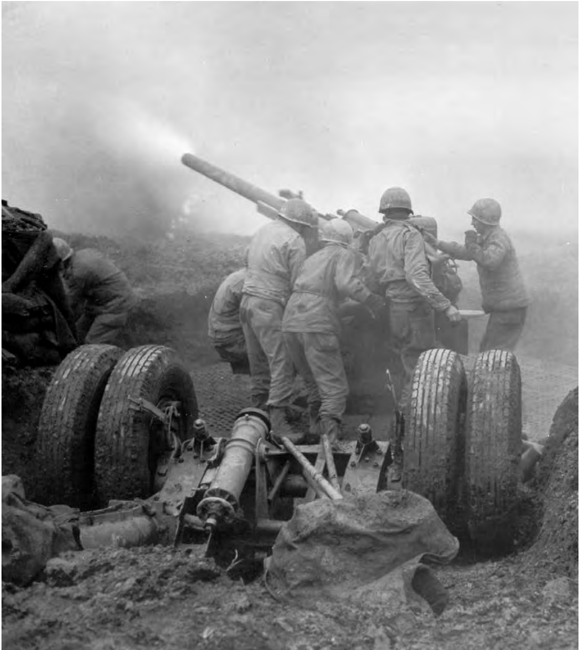
90-MM. ANTI-AIRCRAFT GUN M1 being fired at a German flying bomb passing over Belgium. Liege was subjected to an attack by these robot bombs and suffered considerable damage. Because of the great speed of these weapons it was difficult to combat them, but later with the utilization of the newly developed proximity fuse, the seriousness of the threat of the flying bombs diminished.
